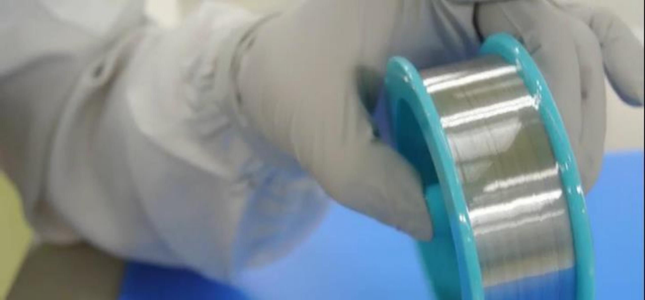
③ Pick the tip of the remaining wire with tweezers and unwind it.
