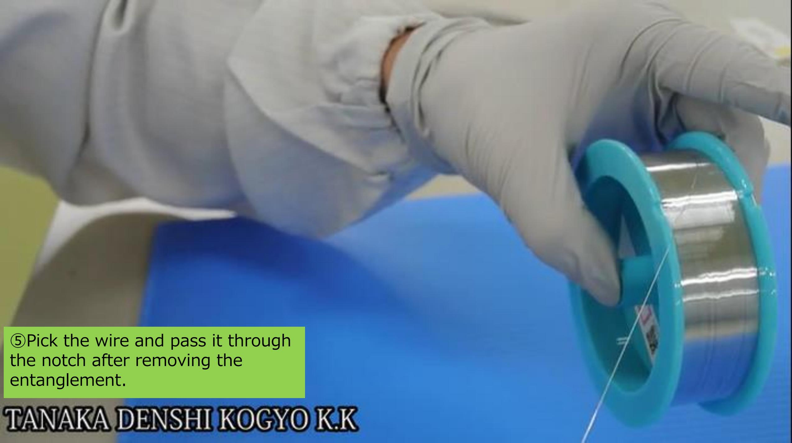
⑤ Pick the wire and pass it through the notch after removing the entanglement.
