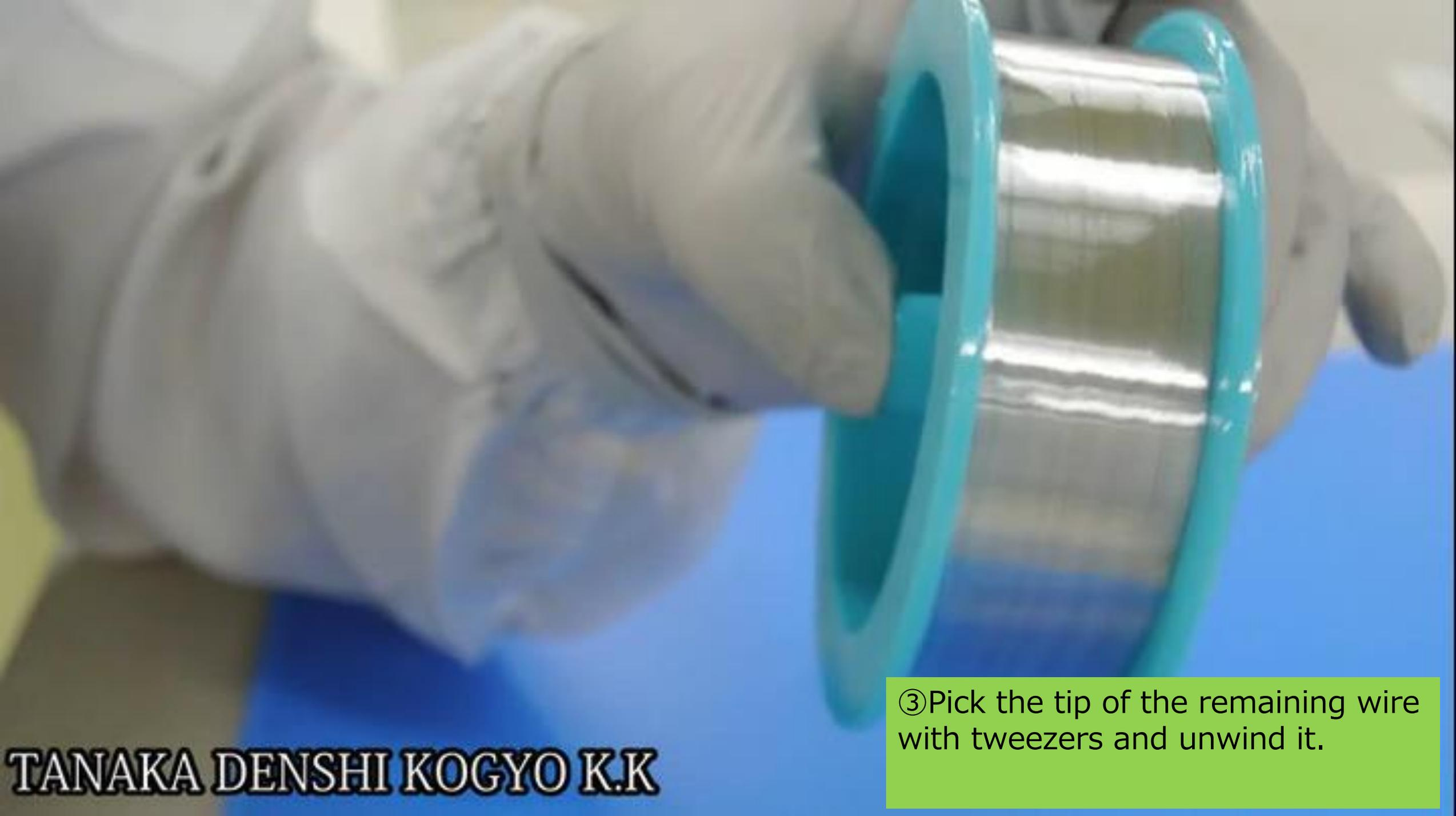
③ Pick the tip of the remaining wire with tweezers and unwind it.
