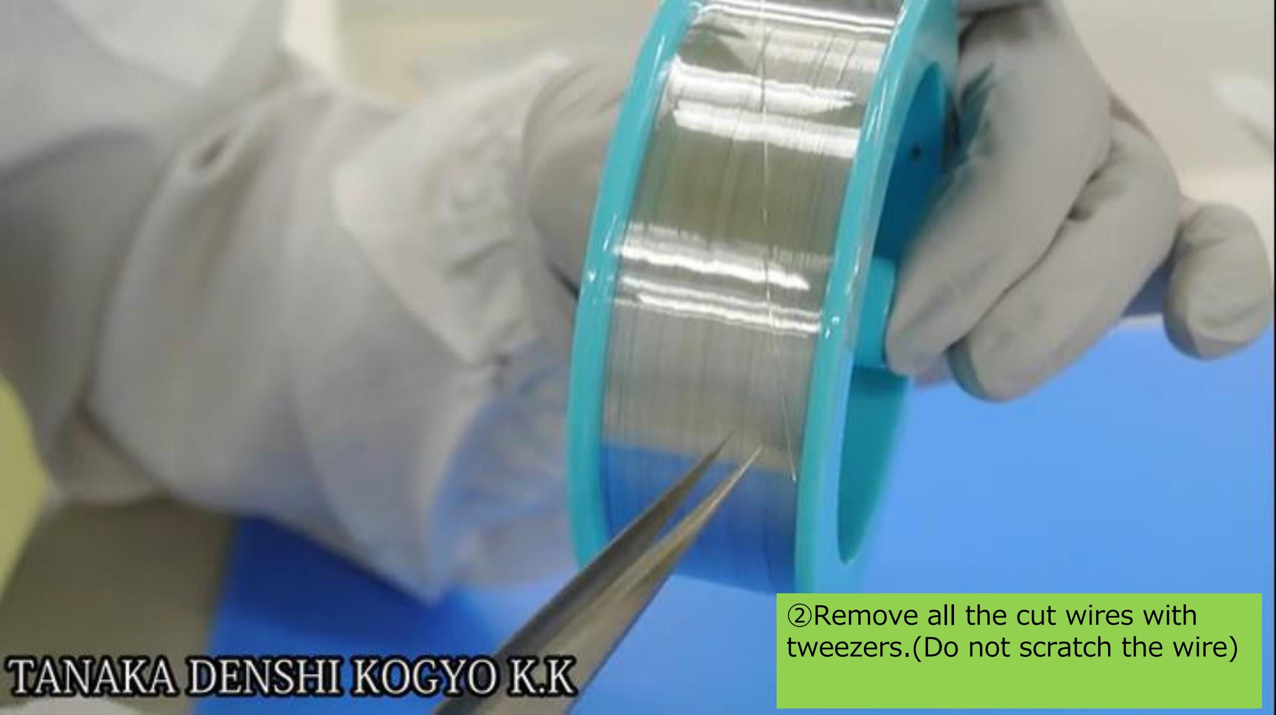
②Remove all the cut wires with tweezers.(Do not scratch the wire)
